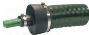
THERMOPEX TERMINATION CAP Rubber end cap provides a watertight seal and protects the insulation from exposure. Simply slip over the end of the pipe and secure with provided clamp.
