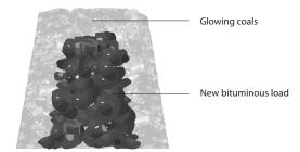
The hot coals are pushed toward the back of the firebox to form a small hill and a valley is created from the hill to the front of the firebox (make sure the valley still has a layer of hot, glowing coals). Bituminous coal is added to the valley making sure it is not too high above the hill at the back of the firebox.
