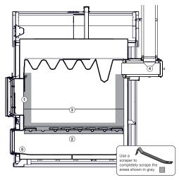
Clean ash and deposits from the areas identified in the order shown. Refer to the corresponding sections for detailed procedures.
