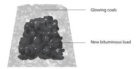
The hot coals are pushed toward the back of the firebox to form a small hill. The remaining hot coals are raked level. Bituminous coal is added in a cone shape on the level coals.
