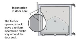
NOTE: If the outdoor furnace is operated with the door open, the firebox door seal may be damaged.
