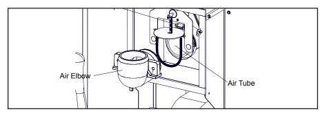
5. Inspect the elbow and clean out any build-up or blockage.
