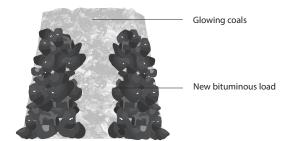
The hot coals are pushed toward the back of the firebox to form a small hill. The remaining hot coals are raked level. Bituminous coal is added in two small strips running from the base of the small hill to the front of the firebox. A strip of hot coals is left exposed down the center. This method works very well when burning run of mine coal containing small fines.
