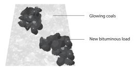
If the coal bed contains a fused, glowing mass of coal, or if there are still large amounts of unburned coal, this method allows you to add coal without disturbing the larger chunks. Use a shovel to add bituminous coal on any exposed cracks or openings in the coal bed. This method can be done with fines, run of mine coal or nut-size coal.
