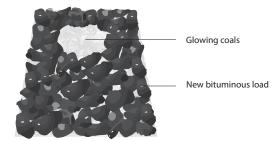
This method is ideal for small and frequent loading. For this method, the coals are first raked even and flat. A thin layer of bituminous coal is added over the whole coal bed, leaving a small area of glowing coals toward the back of the firebox exposed.
