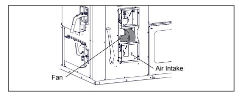
NOTE: Some furnaces use a permanently sealed fan and others use a fan with oil locations. If the fan in your furnace has oil locations, at the end of each heating season oil the combustion fan bearings using the following procedure.
