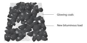
This method works very well when burning run of mine coal containing small fines, or to burn surplus coal fines. It takes advantage of the swell factor that is common with many types of bituminous coal.
